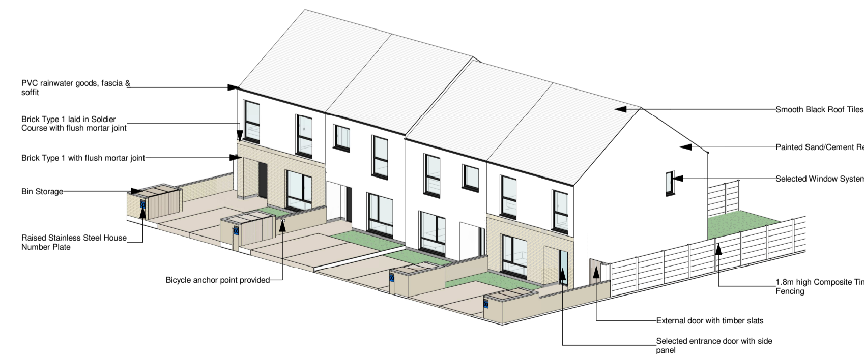
9 House Block HB4 - Axonometric View
